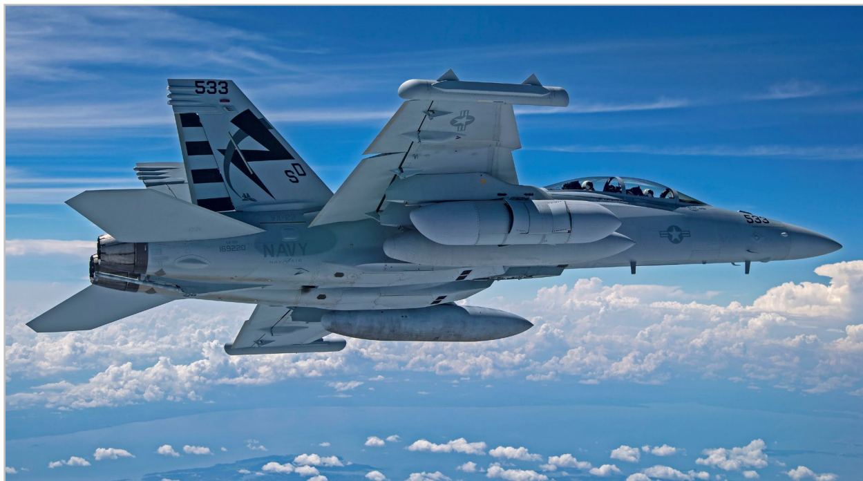
Next Generation Jammer Mid-Band flies for the first time on an EA-18G Growler, Naval Air Station Patuxent River, MD
