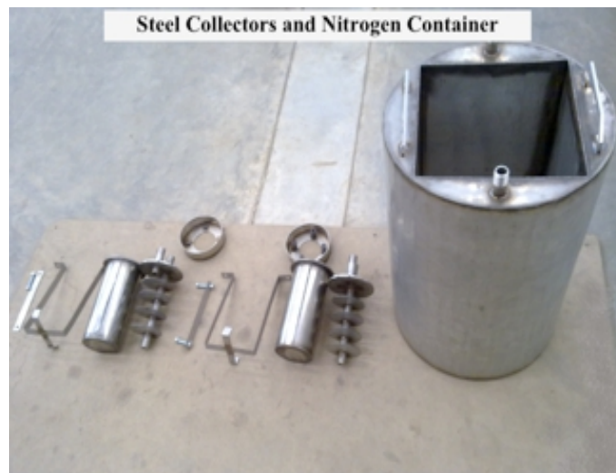
Figure 19. Possible cold trap assembly for collecting UF 6 gas
