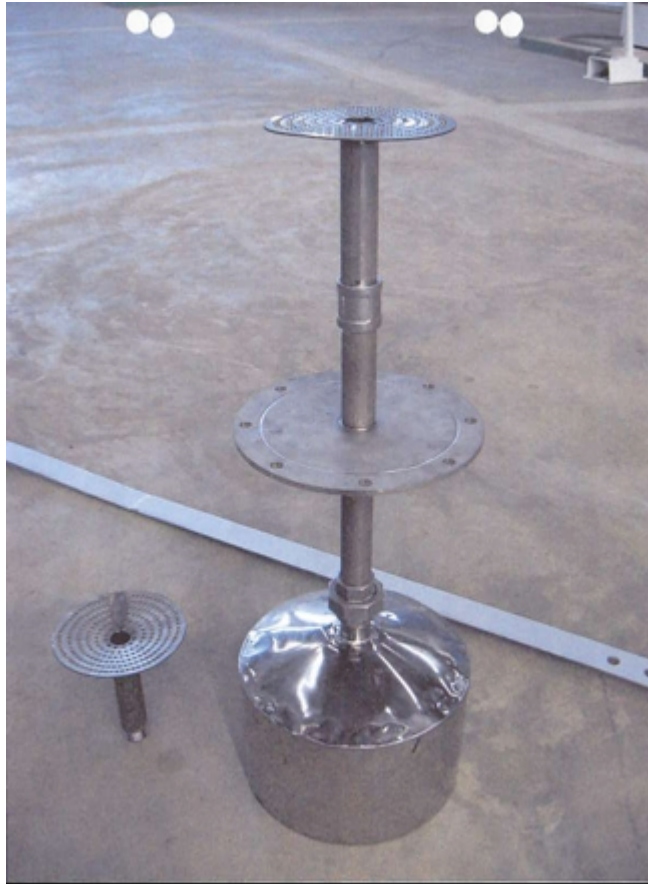
Figure 16. Internal components of the “Fluoride Bed Reactor”
