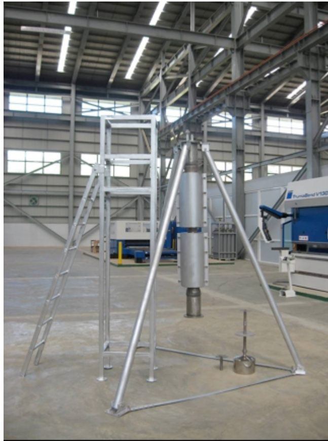
Figure 15. The “fluoride bed reactor” assembly. Note the Trumabend V-130 machine on the right and the Trumatic L 3030 laser cutting machine in the background and compare to Figure 6, the shop layout of Factory 1.
