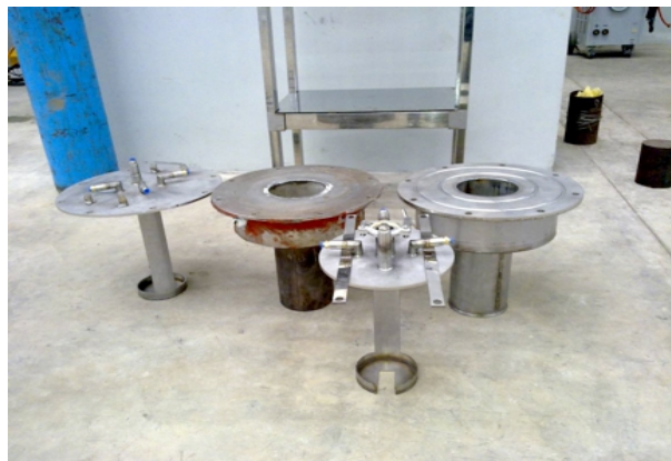
These are ‘bomb reactors’ likely used to convert uranium compounds into uranium metal for bomb or reactor fuel (DVB)
